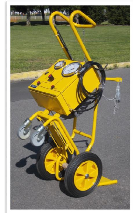
Banc de rinçage hydraulique – *hydraulic rincing cart for Rafale Aircraft*
