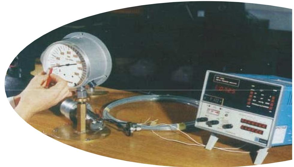
*Cylinder recertification station for periodic inspection of high pressure cylinder
