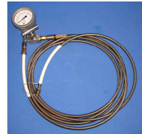
oxygen tightness control test
