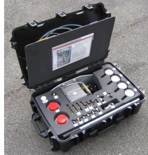
Test unit AIR /hydraulic. Nato case
