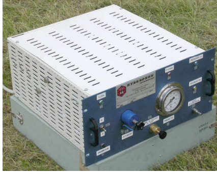
Pressure and temperature cycling unit (for ATEX area) Ethernet controlled (ICS CONSULTANTS)
