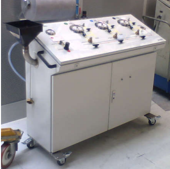
Cleaning unit for space components
