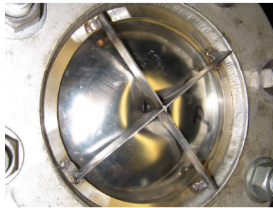
Test on Reverse bursting disc
