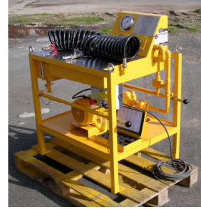
Cleaning unit for RAFALE components
