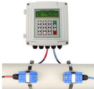
*This instrument is composed by an ultrasonic transducer so the flowmeter can measure the velocity along the path of emitted beam of ultrasound by averaging the difference of transit time between the pulse*
