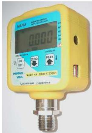
MANU-4A and MANU-5A are digital pressure gauges recommended built with new generation chipset. They are built around an analog part enabling a large time stability associated with a converter enabling internal resolution of 65000 divisions. MANU-4A and MANU-5A digital pressure gauge have an internal
